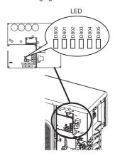
2. Turn on the circuit breaker to supply electricity. In the initial LED display status, D805 is lighted as below.
