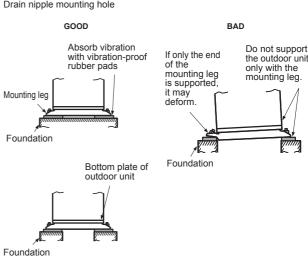
Support the bottom surface of the mounting leg that is in contact with and underneath the bottom plate of the outdoor unit
