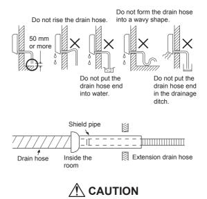
Arrange the drain pipe for proper drainage from the unit.
