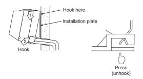
• For detaching the indoor unit from the installation plate, pull the indoor unit toward you while pushing its bottom up at the specified parts.
