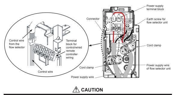
Confirm that every wires are stored in the electric parts box without getting caught before attaching the terminal cover.
