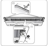
2. Pull out the Air filter. Grab the Air filter and lift it upwards while pushing slightly, and then pull the Air filter forward.
