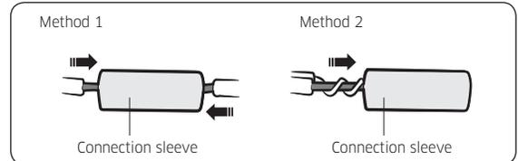
4 Using a crimping tool, compress the two points and flip it over and compress another two points in the same location.
