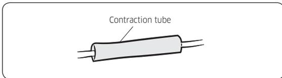
7 After tube contraction work is completed, wrap it with the insulation tape to finish.
