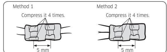
5 Wrap it with the insulation tape twice or more and position your contraction tube in the middle of the insulation tape.
