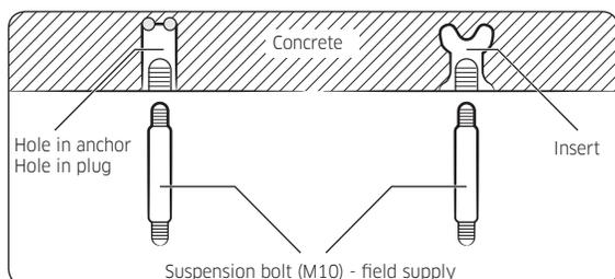
4 Install the suspension bolts, depending on the ceiling type.
