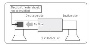
Do not install the electronic heater in the flow channel of the indoor unit fan.
