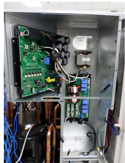
▶ Separate double layer structure of C/Box after remove 3 screws and connector.
