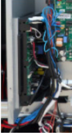
► Comp Wire fix by Holder Wire.
