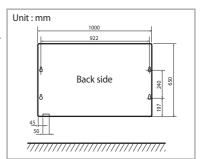
Drill holes for anchor bolts according to the distance 2 and mount them.
