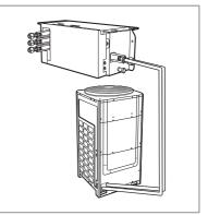
3 Connect the "OUT" refrigerant pipe to each indoor unit (A, B and C).
