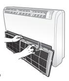
4. Clean the Air filter with a vacuum cleaner or soft brush. If dust is too heavy, then rinse it with running water and dry it in a ventilated area.
