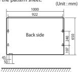
3. Install the unit onto the ceiling. Be sure to arrange the drain hose so that it is leveled lower than the drain hose connecting port of the indoor unit.
