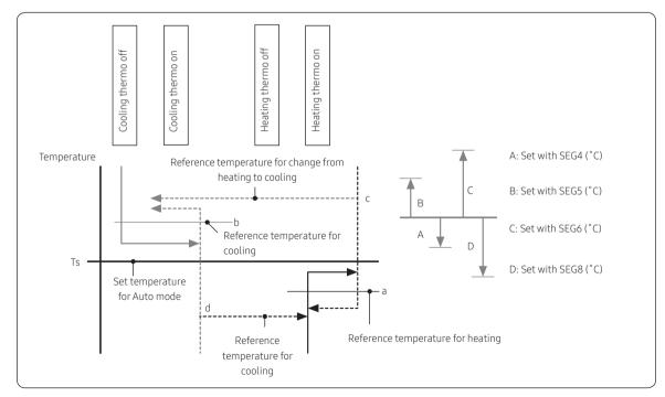
The mode change between the Cool and Heat modes is made only when the thermo off state is maintained for the period of time set with SEG9.
