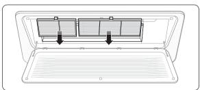
Pull the air filter out of the indoor unit
