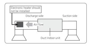
Do not install the electronic heater in the flow channel of the indoor unit fan.
