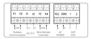
\* The output of hot coil terminal is AC 220 V / 230 V (The same as Indoor Unit's input Power)
