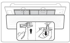
Press the **Push** signs on the air filter. Grab the handle of the air filter and pull it out from the indoor unit.
