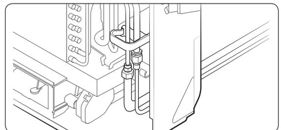
7 Hanging the indoor unit on the Bracket Hanger, then fix the Indoor Unit by using 4 Screws.
