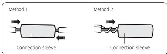
4 Using a crimping tool, compress the two points and flip it over and compress another two points in the same location.
