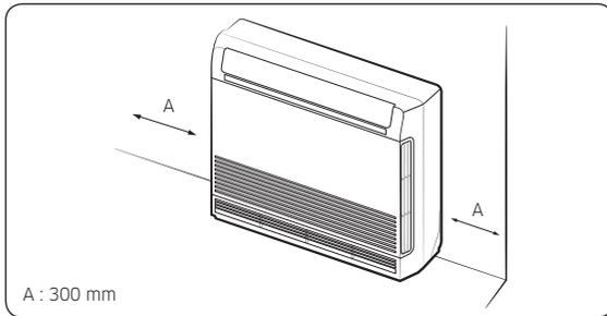
2 When you install the indoor with side-pipe connection, please make space more than 300mm from the wall.
