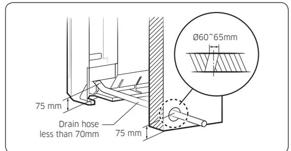
6 The pipes & cable should be gone through the bottom back hole.
