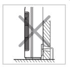
The hose must NOT slant upwards.
