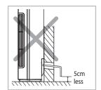
Keep a clearance of at least 5cm between the end of the hose and the ground.
