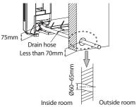
**6.** The pipes & cable should be gone through the bottom back hole
