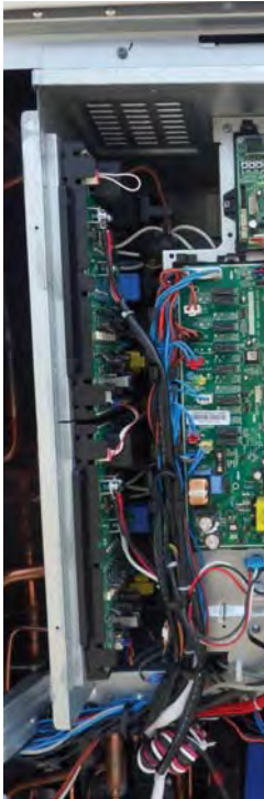
► Comp Wire fix by Holder Wire.
