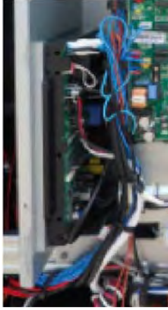
► Comp Wire fix by Holder Wire.
