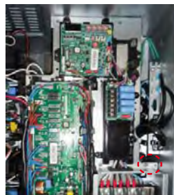
► Separate double layer structure of C/Box after remove 3 screws and connector.
