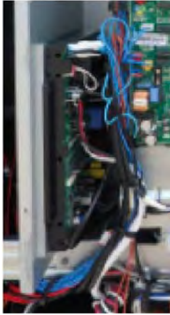
► Comp Wire fix by Holder Wire.
