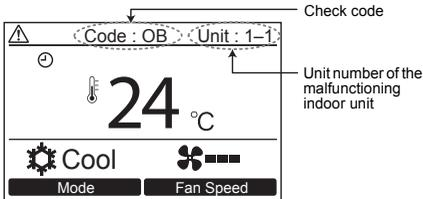
When an error has occurred in the air conditioner, the check code and the unit number of the indoor unit appear on the display of the remote controller.
