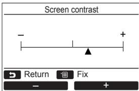
**1** Push the [▲ ▲] / [▼ ▼] button to select "3.Screen contrast" on the "Initial setting" screen, then push the "Set" [F2] button.
