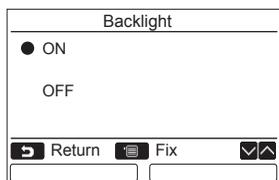
**1** Push the [ ] / [ ] button to select “4.Backlight” on the “Initial setting” screen, then push the “ Set” [ F2] button.
