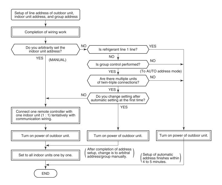
• When the following addresses are not stored in the neutral memory (IC10) on the indoor P.C. board, a test run operation cannot be performed. (Unfixed data at shipment from factory)
