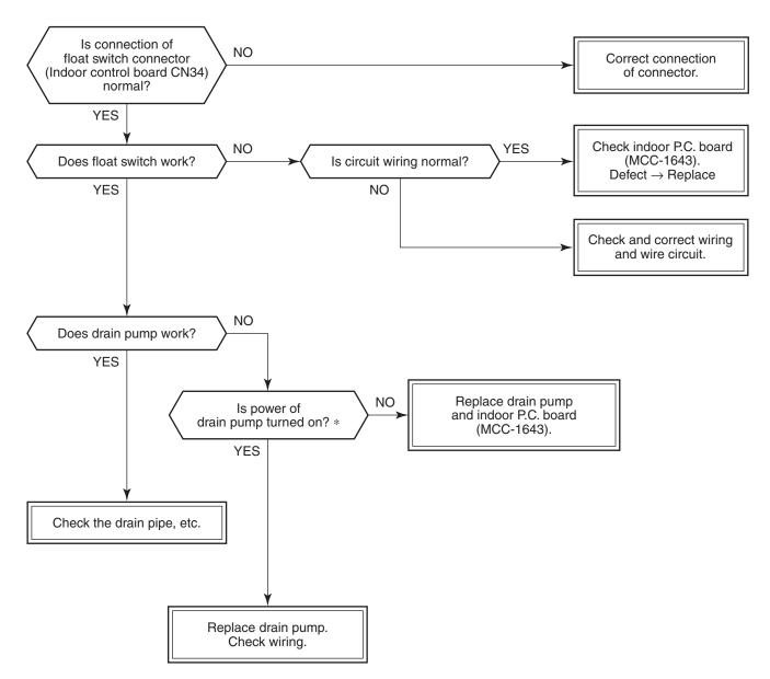
\* Check that voltage of 1-2 pin of CN504 on the indoor P.C. board is +12V. (1 pin is plus (+).)
