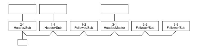
• Master unit: The master unit receives the indoor unit data (thermo status) of the sub (Without identical line address & indoor/outdoor serial) and then finally controls the outdoor compressor matching with its own thermo status.
