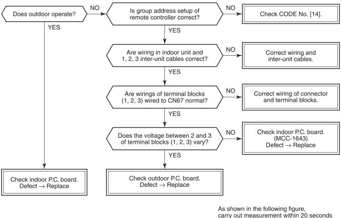
carry out measurement within 20 seconds after the power was turned on.
