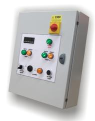
This panel is designed to control two indoor units on a duty standby basis, one unit running while the remaining unit is on standby. Unit one will run for 100 hours, then change over to the standby unit which in turn will run for 100 hours. This pattern will be repeated on a continuous basis.
