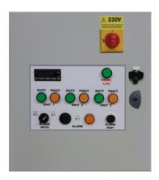
This panel is designed to control Three indoor units on a duty standby basis, two units running while the remaining unit is on standby. Units 1 + 2 will run for 100 hours, then change over to the second set of units (1 + 3) which in turn will run for 100 hours. This pattern will be repeated with (2 + 3) running and so on.
