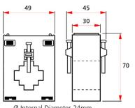
Ø Internal Diameter 24mm Busbar 30x10mm, 20x20mm
