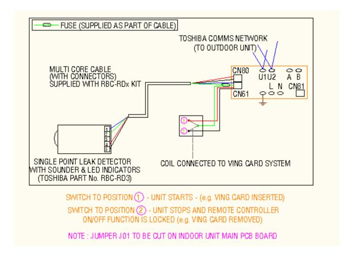
The above drawing shows the Leak detector connected to a VRF indoor unit.
