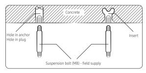
3 Install the suspension bolts, depending on the ceiling type.
