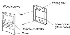
3. Connect the wires from the hydro unit to the remote controller terminal block.(Refer to "Wiring".) Connect the wires of the remote controller following the terminal numbering convention of the indoor unit to prevent miswiring. (Do not apply AC 230V mains voltage to the remote controller as it will be damaged).
