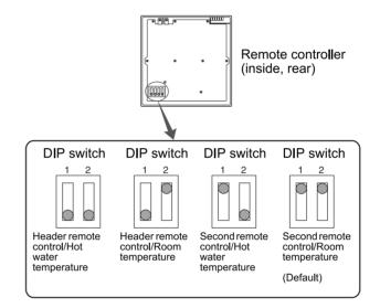
For a dual remote controller system, install the remote controllers in the following way.
