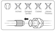
**6** Align the pipes and tighten the flare nuts first manually and then with a torque wrench, applying the following torque.
