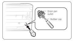
4 Attach the rubber cap with a screwdriver by turning it to the right until it fixes to the end of the groove.
