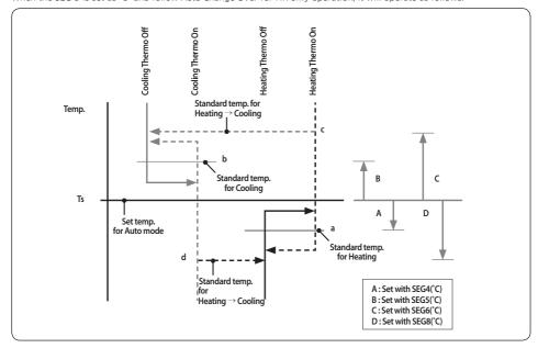
Cooling/Heating mode can be changed when Thermo Off status is maintained during the time with SEG9.
