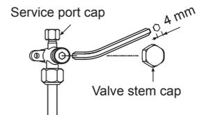
5. Tighten the service valve stem cap and service port cap securely.
