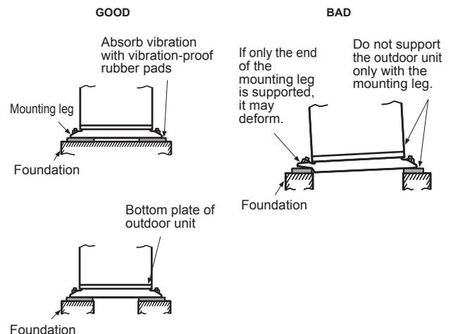
Support the bottom surface of the mounting leg that is in contact with and underneath the bottom plate of the outdoor unit.
