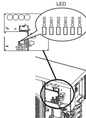
2. Turn on the circuit breaker to supply electricity.
