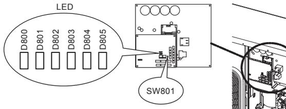
3. Hold down SW801 for at least 5 seconds, and check that D800 is lighted and D804 light is flashing(1time/sec.).
