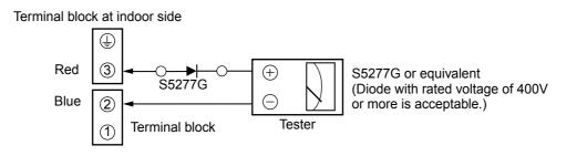
Normal time : Voltage swings between DC15 and 60V. .....Inverter Assembly check (**11-8-1**.) Abnormal time : Voltage does not vary.
