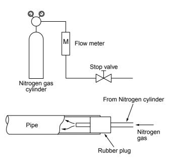
Fig. 3-5-1 Prevention of oxidation during brazing
