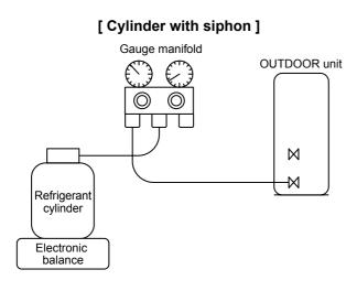
R32 refrigerant is HFC mixed refrigerant. Therefore, if it is charged with gas, the composition of the charged refrigerant changes and the characteristics of the equipment varies.
