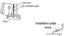
• For detaching the indoor unit from the installation plate, pull the indoor unit toward you while pushing its bottom up at the specified parts.
