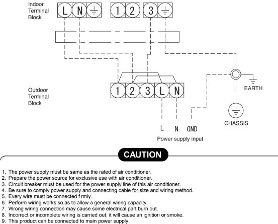
This product can be connected to main power supply. Connection to fixed wiring : A switch which disconnects all poles and has a contact separation at least 3mm must be incorporated in the fixed wiring.
