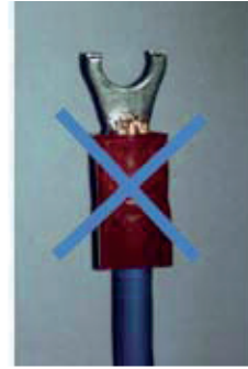
Terminal has been cut.
