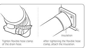
When passing the drain hose through the hole drilled in the wall, check that none of the following situations occur:
